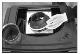
**Figure 8.4** Install the inner flue collar <u>on rear of appliance</u>, with damper rod pointing up. A dab of high temperature silicone on the gasket will help gasket adhere to the appliance.
